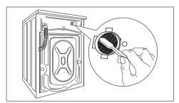
Screw the hose back to the machine and make sure the connection is tight. 8. Turn on the water tap.
